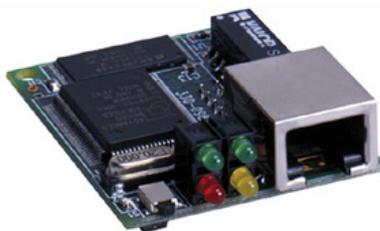
The CoBox Micro is designed to work with the SSP-C and SSP-E legacy controllers. The drawings below illustrate the location of the CoBox Micro for each type of controller.
