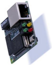
The GIPRCNX has four status LEDs: serial port (Channel) 1 status, serial port (Channel) 2 status, diagnostics, and network link status. See the following table for a complete description of status LED pin out location and function.
