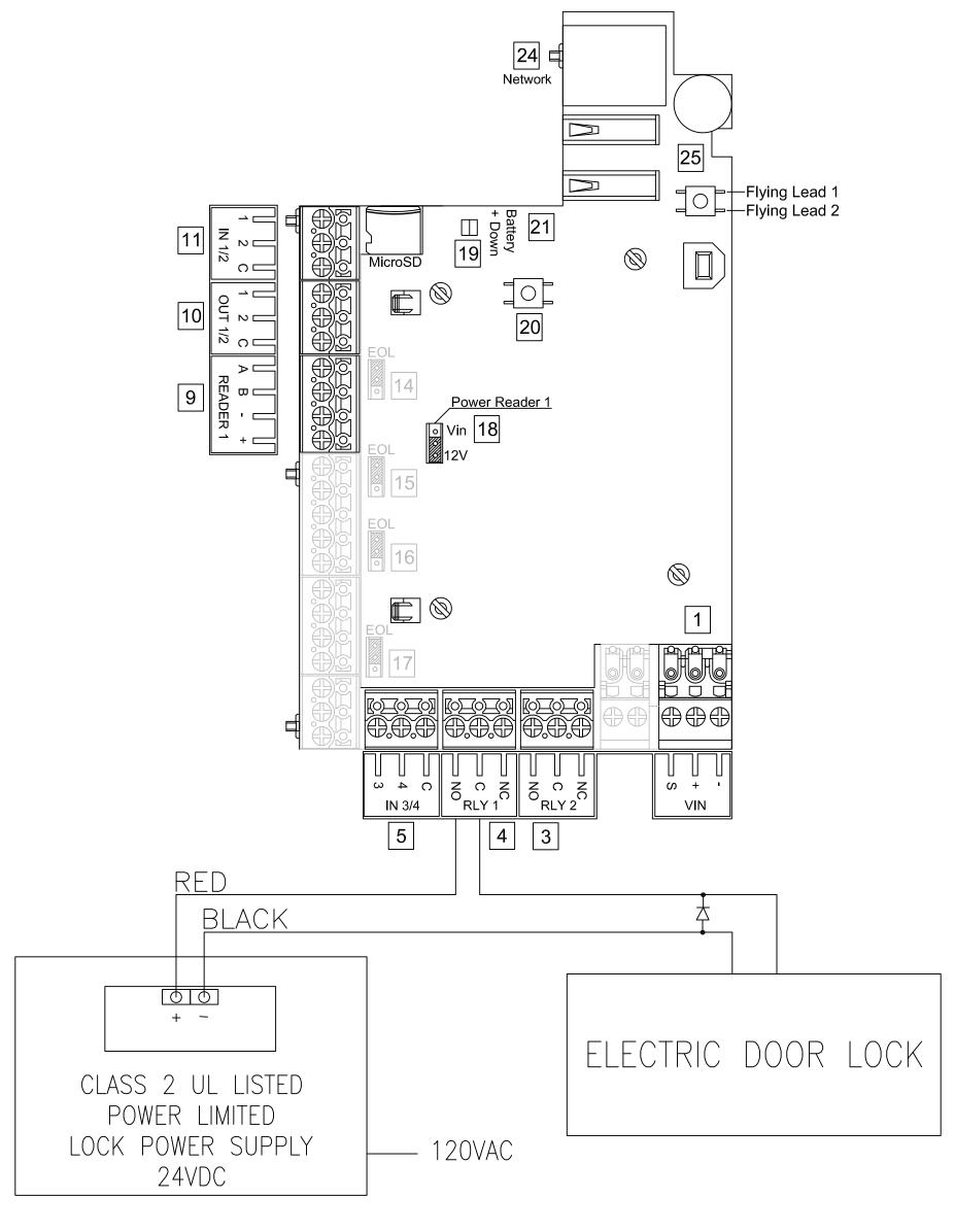
THE LOCK IS WIRED ACROSS 24V AND COM. A OV LINK TO COM IS THEN REQUIRED TO COMPLETE THE CIRCUIT. THIS WILL BE WIRED TO NO OR NC DEPENDING ON THE LOCK TYPE: FAIL OPEN / FAIL CLOSED. (ABOVE DIAGRAM IS OF FAIL OPEN).
