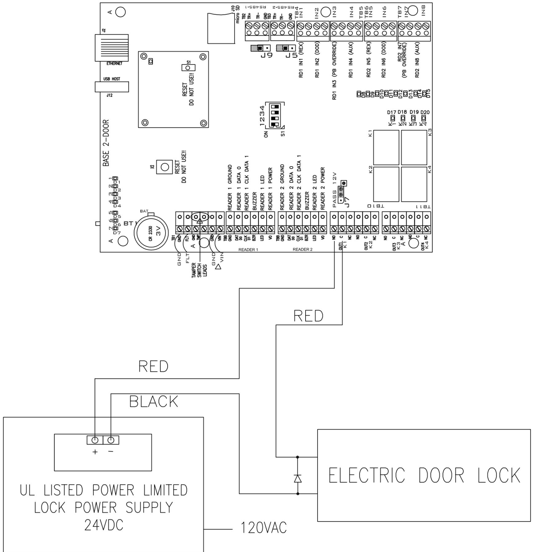
A DIODE IS USED TO ELIMINATE THE VOLTAGE SPIKE SEEN ACROSS AN INDUCTIVE LOAD WHEN ITS SUPPLY VOLTAGE IS SUDDENLY REMOVED.
