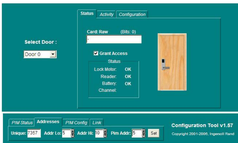
Example address settings for the second of two PIMs on one channel
